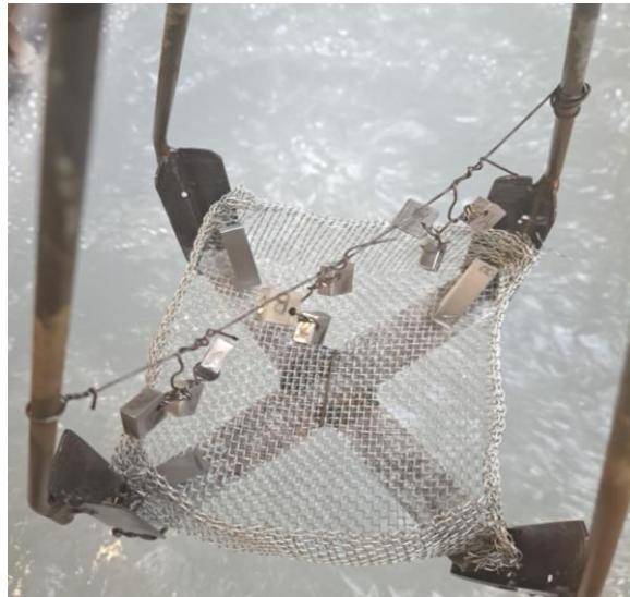
Fig 1 Immersion of components in a boiling alkaline salt solution
