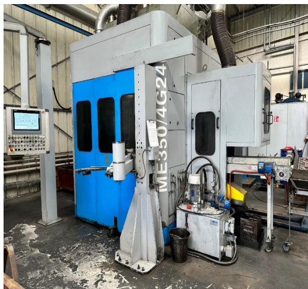
Fig. 4 Automatic forging station for brass slide blocks at FAS – MECOLPRESS 350 hydraulic press
