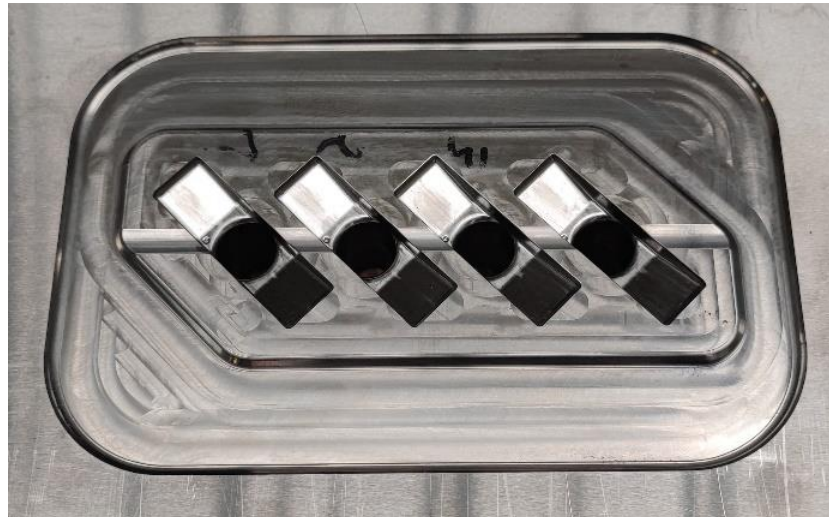
Fig. 6 View of the multi-cavity for the slide blocks in the lower die for automatic forging process
