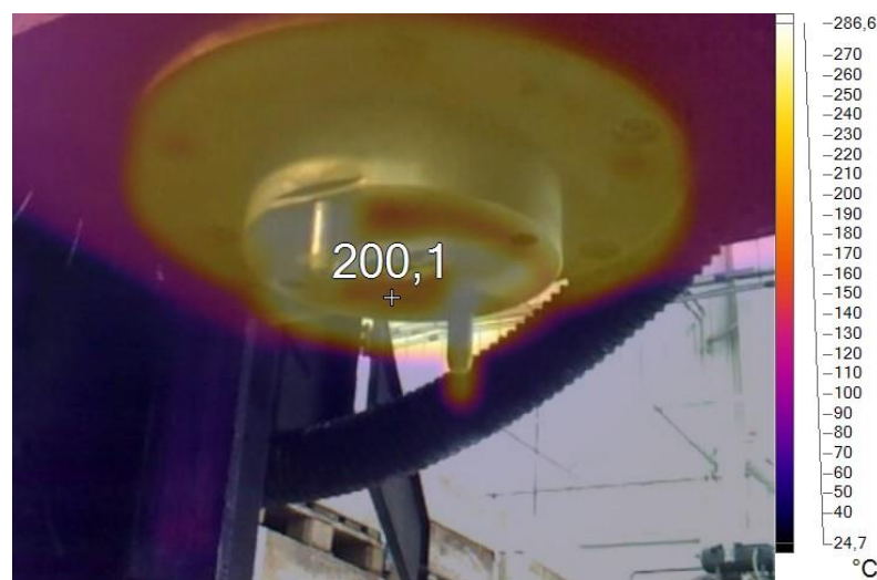
Fig. 7 Temperature value prior to the start of the manual forging process for the upper die
