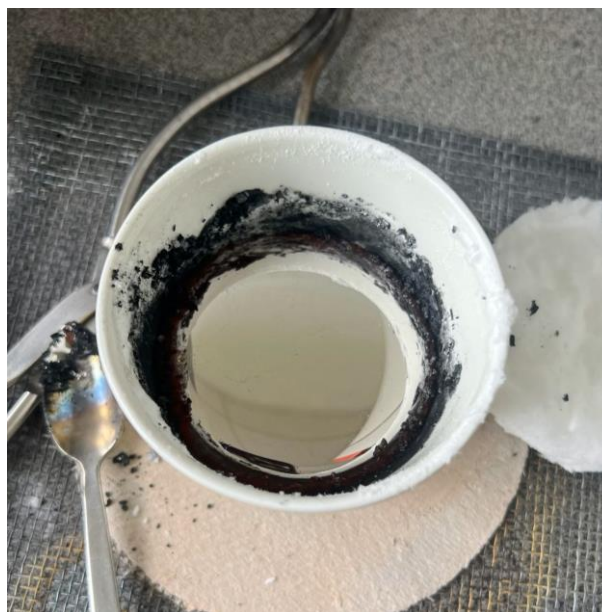
Fig. 2 Sn-P alloy after melting process.
