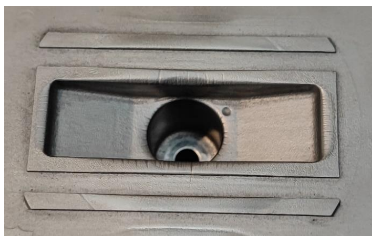
Fig. 5 View of the single cavity for the slide block in the lower die for manual forging process
