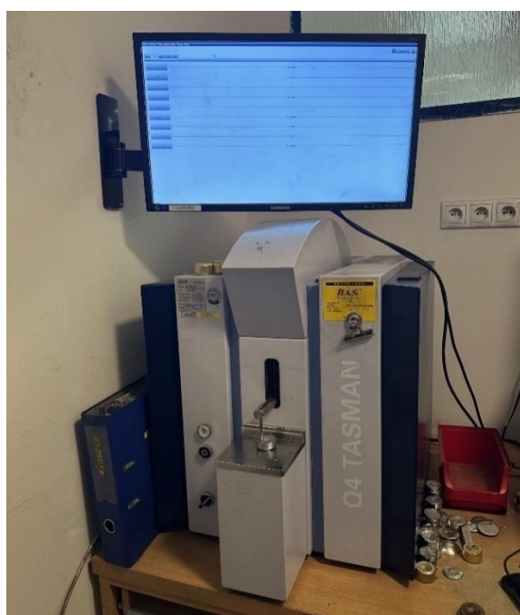
Fig. 3 Digital optical emission spectrometer Q4 TASMÁN with a CCD detector
