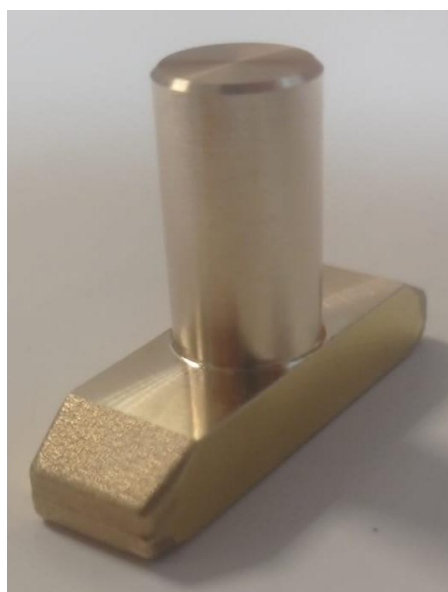
Fig. 2 Slide block after final machining operation
