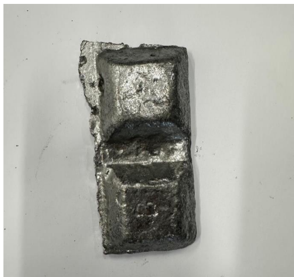
Fig. 4 SnP2 alloy in waffle shaped ingots
