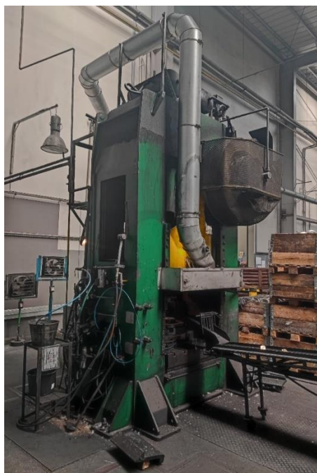
Fig. 3 Manual forging station for brass slide blocks at FAS – MECOLPRESS 350 mechanical press
