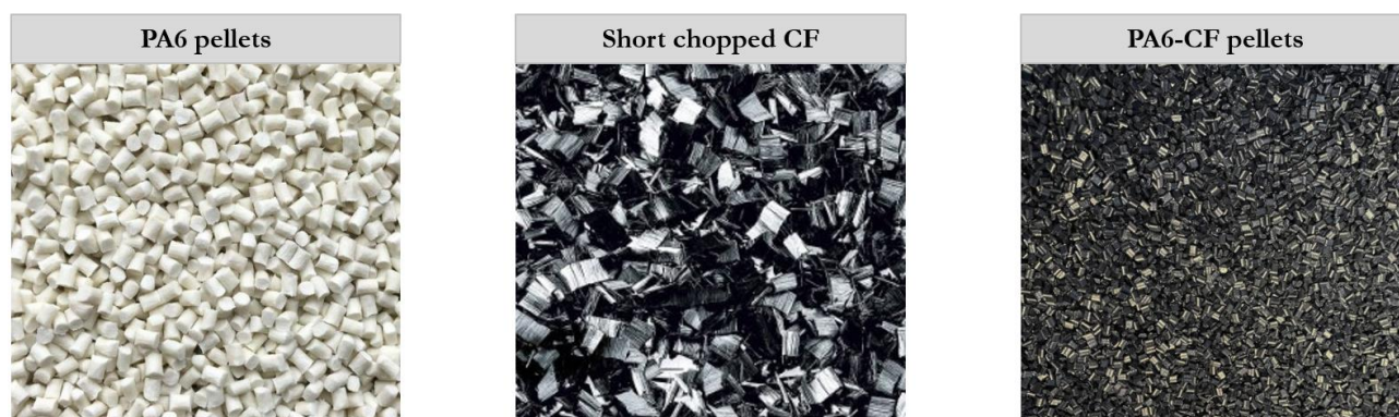
Fig. 1 Examples of PA6 pellets, short chopped CF and PA6-CF pellets
